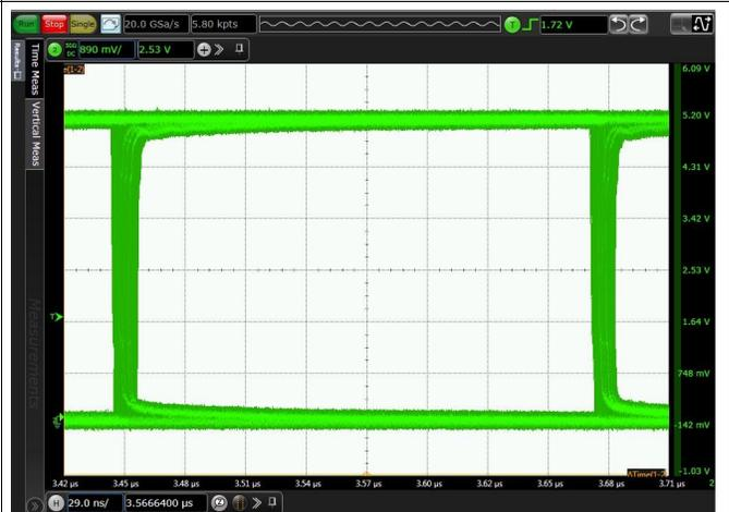
Figure 23. Eye Diagram at 4 Mbps PRBS  $2^{16} - 1$ , 5 V and 25°C
