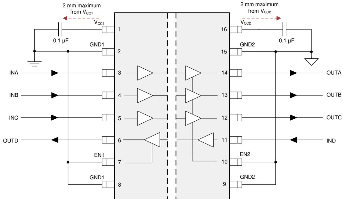
**Figure 19. Typical ISO7041 Circuit Hook-up**
