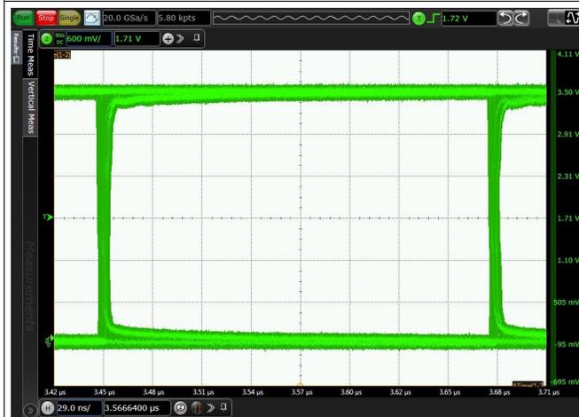
Figure 22. Eye Diagram at 4 Mbps PRBS  $2^{16} - 1$ , 3.3 V and 25°C
