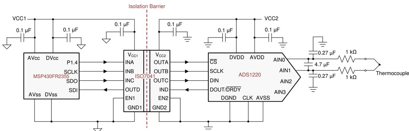
Figure 18. Isolated SPI for a Temperature Field Transmitter
